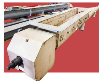
presents significant handling difficulties. To ensure safe and efficient downstream operations, this material needed to be cooled to 400°F. Our solution was a custom-designed cooling screw, featuring a jacketed design that circulates 90°F water. This innovative system not only achieves rapid heat dissipation but also protects the integrity of the equipment and ensures smooth material flow.
